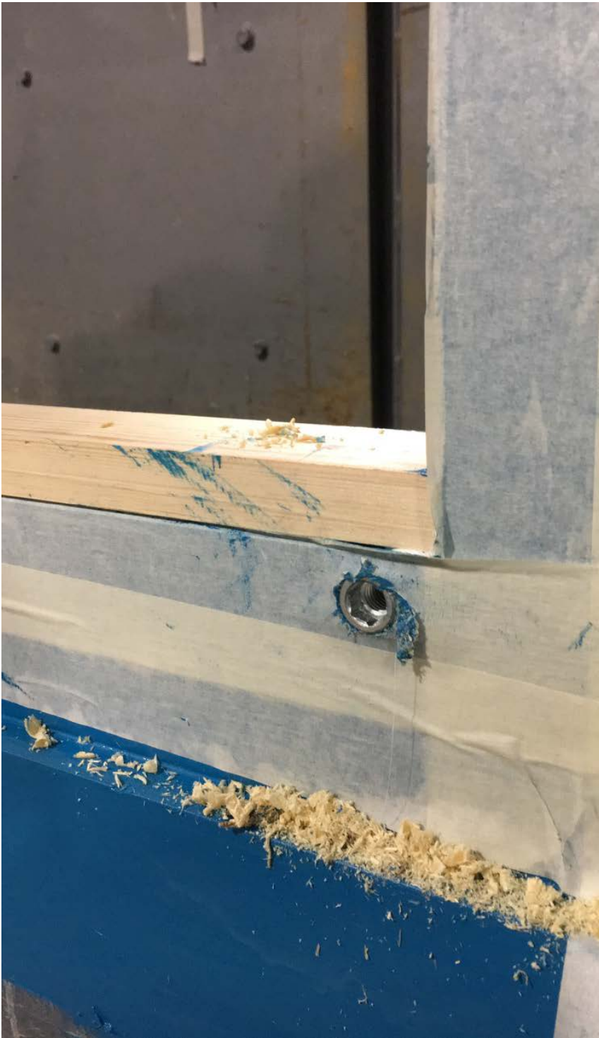
Figure 1.2: Threaded 'rivnuts' used to mount product to frame.
