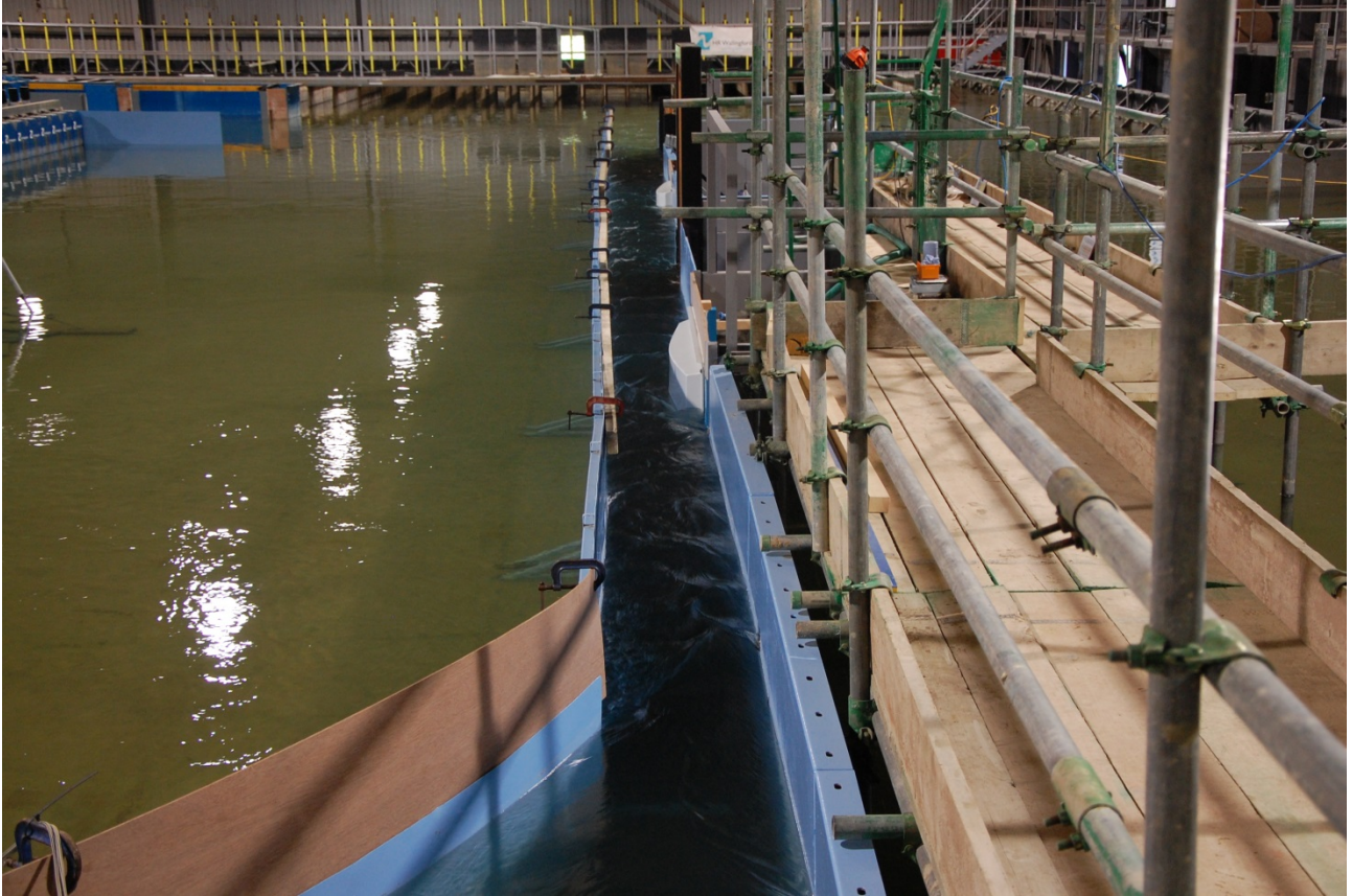
Figure 3.3: Current testing setup showing wave guide positions and flow direction.
