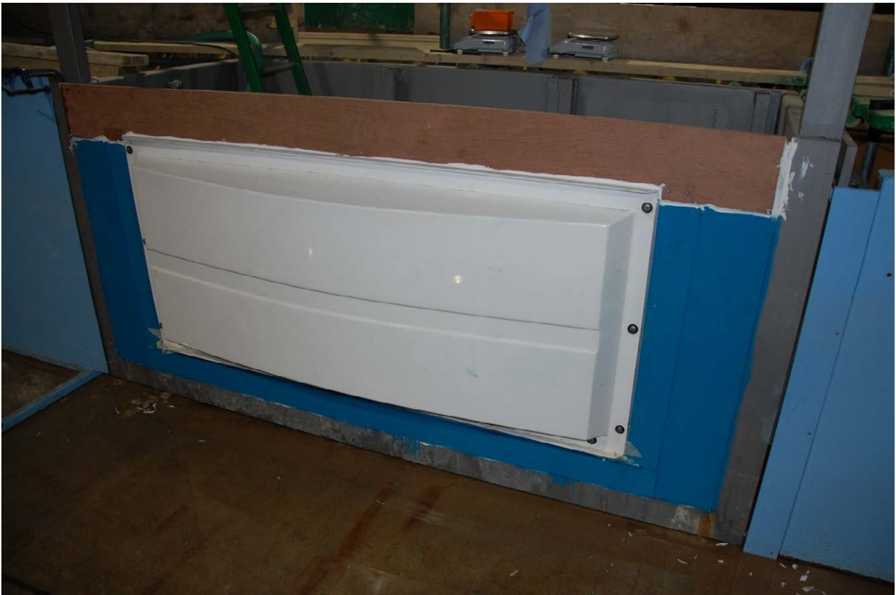
Figure 1.4: Plywood attached above product to prevent overtopping from wave overtopping.
